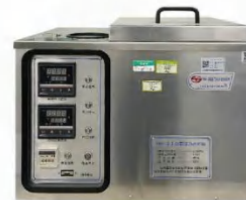
沥青压力老化箱 Asphalt pressure aging box
