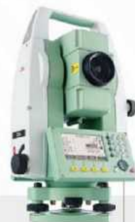
徕卡TS30全站仪/超站仪 Leica TS30 total station instrument / super station instrument
