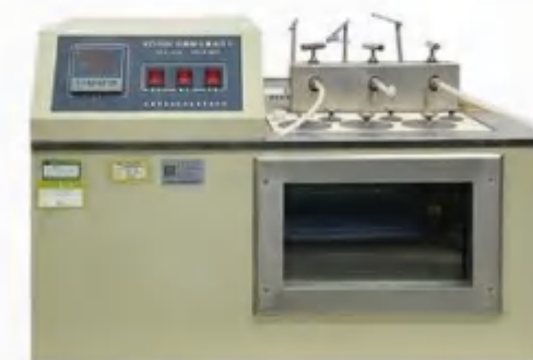
沥青蜡含量测定仪 Asphalt wax content tester
