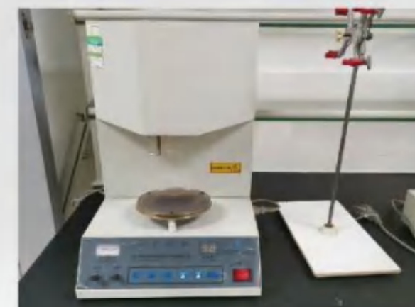
水泥游离氧化钙快速测定仪 Rapid Measuring Instrument for Free Calcium Oxide of Cement
