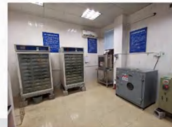
恒温水养护箱沸煮箱恒温干燥箱 Constant Temperature Water Maintenance Box Boiling Box Constant Temperature Drying Box
