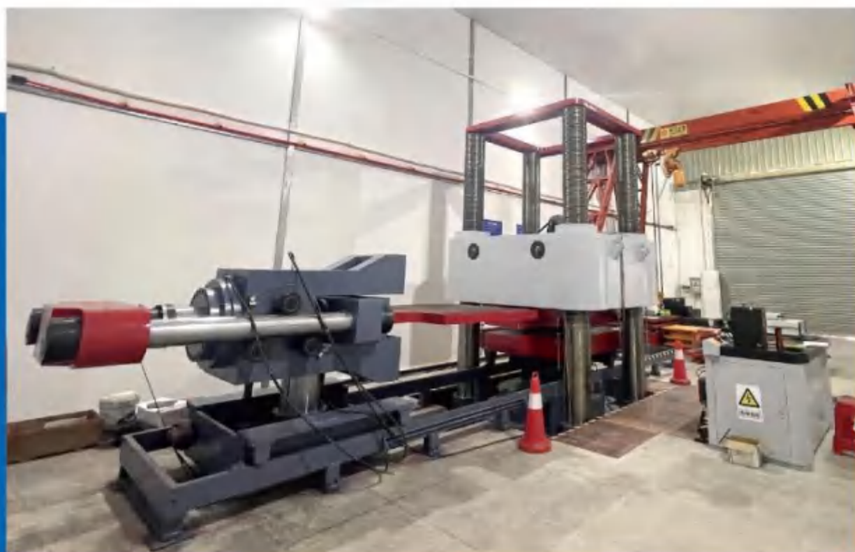
2000吨橡胶支座压剪试验机 2000 T rubber bearing compression shear testing machine
